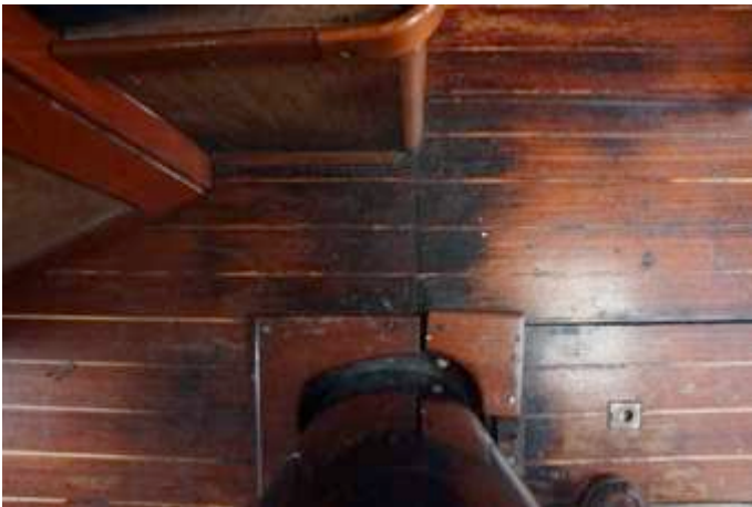
To starboard of the keel stepped mast. Totally stained by bilge contents over many years.
