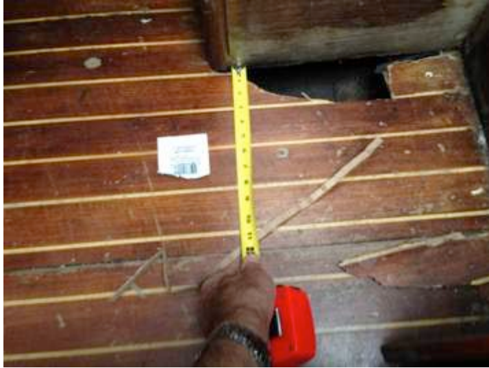
The floor below the chart table... \frac{1}{4} " thick ply that had totally rotted through with the help of a crew member's foot.
